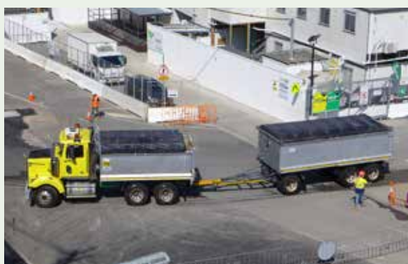
Figure 24: Loads containing demolition material, soil, sand or excavated material must be fully covered before entering the road network (see 3.14 ).
