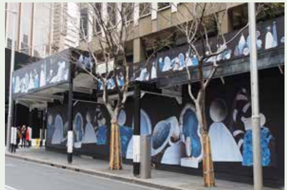
Figure 3.11: Clear column spacings of not less than 4.0 metres is required in the city-centre (refer to map at Figure 1.1a ) however, this can be varied for special site-specific needs (see Figure 3.12 ) and steeply sloping footways .
